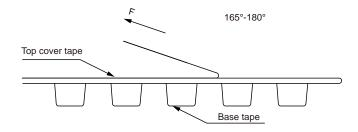
The peel force of top cover tape shall be between 0.1 to 0.98 N
