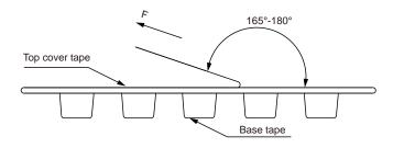
The peel force of top cover tape shall be between 0.1 to  $1.3\,\mathrm{N}$
