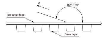
The peel force of top cover tape shall be between 0.1 to  $1.3~\mbox{N}$
